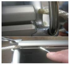
Round the ends of the long ropes and insert into the sail cover grooves in the top of the boom shell. Use a sharp tool such as an ice pick or awl to pull the ropes through the grooves to the front of the boom. Pull the sail cover through to the front of the boom.
