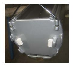
If the existing sail cover is sufficiently intact, it can be used to pull the ropes of the new cover through the boom. This should be considered prior to removing. After removing the aft cowl ensure that the sail cover guides are clean and fair.
