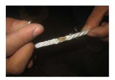
Sewing back and forth at four places around the joint will keep the joint from becoming too bulky.
