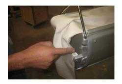
Super Lube or similar product added at the sail cover guides and top corners of the boom shell is necessary to reduce friction and ensure smooth operation.
