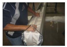
Once the new sail cover is installed, it will feel quite stiff and difficult to operate - this is typical. Deploying and retracting the cover several times will help the sail cover to break in. Further hand pressing of the pleat fold, and additional Super Lube may be necessary. After the new cover has broken in and is properly lubricated, it should operate smoothly and with minimal physical effort.
