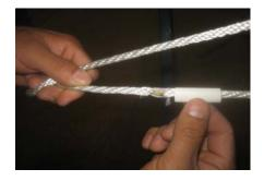
slide the shrink wrap over the joint and use a heat gun to shrink the tube.
