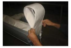
Feed the aft end of the sail cover through the aft guides.
