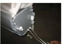
An optional method is to run the snake through one of the holes in the front of the boom, aft, and out the slot in the bulkhead. A messenger line can then be drawn through the boom and tied off tightly. This is then repeated through the other hole, and the new ropes can be pulled through with less chance of twisting.
