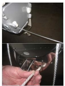
When possible it is advised to use the existing ropes to pull the new ropes through the boom. This helps avoid getting the ropes twisted. Otherwise:
