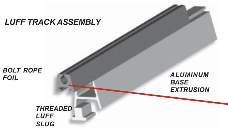
11. The COASTAL Leisure furl uses a two piece base and foil system. The foil portion is an extrusion of UHMW-PE high tensile polymer. After mounting the aluminum base extrusion, with the .020 space as shown below, slide on the foil. The foil pieces can simply be joined by butting them together. Due to thermal expansion of the polymer bolt rope foil; a gap of 1" must be left between the top end of the foil and the bottom of the halyard sheave box.
